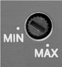
Figure 3-16 Equalize 1 Battery Charger Rate Potentiometer (Position "1")
